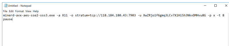
Fig. 228: Notepad file showing an example command to start a CPU miner
